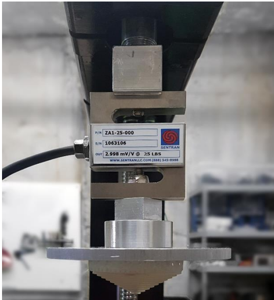
Figure 3: Separation force test rig assembly
