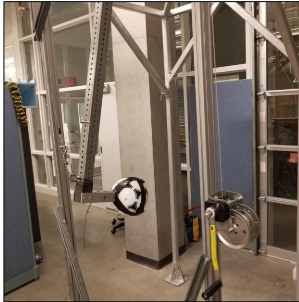
Figure 1: Completed pendulum impactor system
