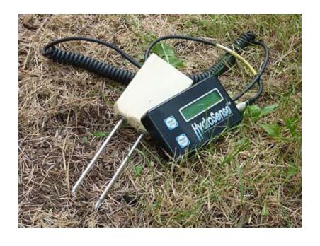
The velocity of propagation used to calculated volumetric water content which is displayed on the LCD (or recorded on a data logger)
