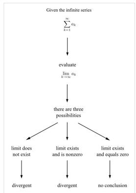
This diagram shows the steps involved in conducting the divergence test. Observe that in the case that the limit equals zero, the test does not tell us if the series is convergent or divergent (other convergence tests can be employed in this case). This is an area that is a common source of confusion among calculus students.
