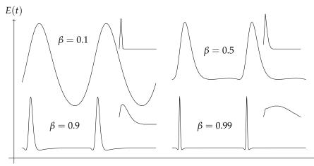
Figure 15: Electric field from a gyrating particle  $\beta = 0.1, 0.5, 0.9$  and 0.99. The insets show the power spectrum with  $\omega/\omega_c$  along the x-axis. These were calculated without the small-angle or ultrarelativistic approximations. Keep in mind a particle with  $\gamma = 10^3$  has
