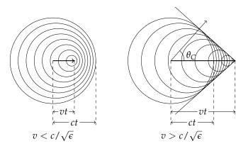
Figure 7: The propagation of electromagnetic waves from a source travelling slower and faster than the speed of light in the medium  $(c/\sqrt{\epsilon} \text{ in } \S$  ).
