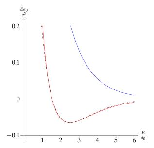
Figure 19:  $E_u$  (upper curve) and  $E_g$  (lower curve) for  $H_2^+$ . The dashed curve is a well-fit Morse potential for  $E_g(R)$ .
