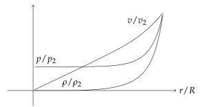
Figure 29: Variation of the density, velocity and pressure behind the shock for the Sedov-Taylor blast wave
