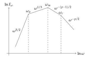
Figure 17: Complete synchrotron spectrum for an age less than the maximum cooling time (slow cooling).
