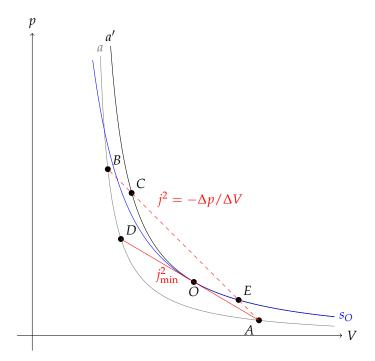
Figure 30: Shock (Hugoniot) Adiabat (in gray), Detonation Adiabat (in black) and Standard (Poisson) Adiabat (in blue)
