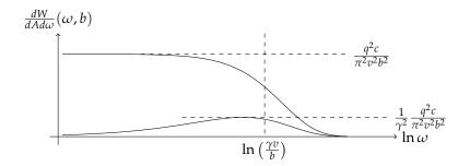
Figure 12: The frequency spectra for the electric field in the *y*-direction (upper) and x-direction for a fast moving charge
