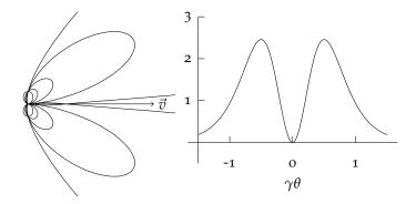
Figure 6: Radiated power as a function of angle and  $\gamma\theta$  for longitudinal motion. The left-hand panel shows from inside out  $\beta=0,0.2,0.4,0.6,0.8$ .
