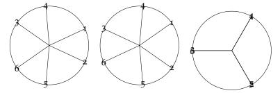
Because we are only interested in the x-coordinate (the cosine of the angle), we see that solutions 1 and 2, 3 and 6 and 4 and 5 are equivalent, so we only need to keep the solutions with t between zero and  $\pi$ . In the left diagram we used  $t=25^{\circ}$  so we only have a single value with cos t greater than zero. We can discard negative values of cos t because that would yield that the surface of the water lies underneath the surface of the bottom.
