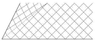
Figure 27: The Characteristic Structure for a Compression Wave, a > 0. Notice the abrupt transition between the regions.
