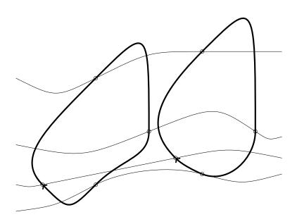
Figure 24: The circulation around a close contour (bold lines) that travels with the fluid along the streamlines (light lines) is conserved if the fluid is isentropic.
