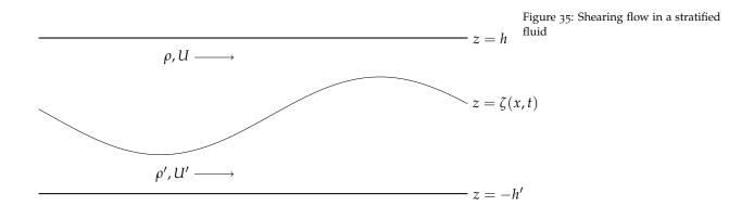
Let's imagine a different type of wave on a fluid. Let's imagine we have two fluids in a gravitational field. The lower fluid has density  $\rho'$ , velocity U' and thickness h' and the upper fluid has density  $\rho$ , velocity U and thickness h. Let's have  $\zeta(x,t)$  denote the displacement of the interface in the z-direction. Let's assume that both fluids are incompressible and the flow is irrotational, so we can define
