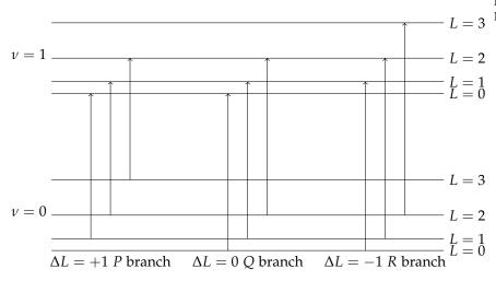
Figure 21: Roto-Vibrational Transitions Neglecting Stretching
