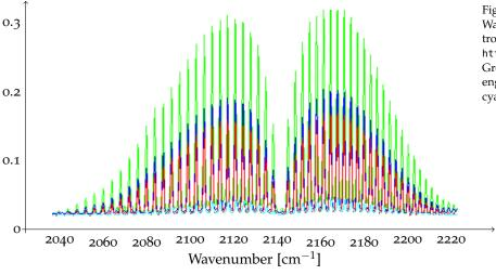
Figure 22: Absorption vs. Wavenumber for FTIR Spectroscopy of CO in car exhaust from http://home.swipnet.se/~w-74877/ftir/ftir.htm. Green is a cold engine, blue is a warm engine, red is a calibration reading and cyan is a 100ppm calibration.
