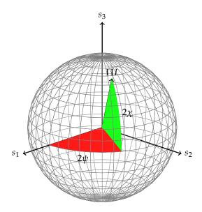
Figure 4: The Poincaré sphere
