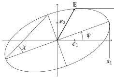
Figure 3: Electric field of linearly (left) and elliptically (right) polarized waves
