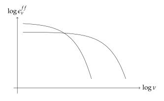
Figure 10: Thermal bremsstrahlung spectra for two temperatures that differ by a factor of ten
