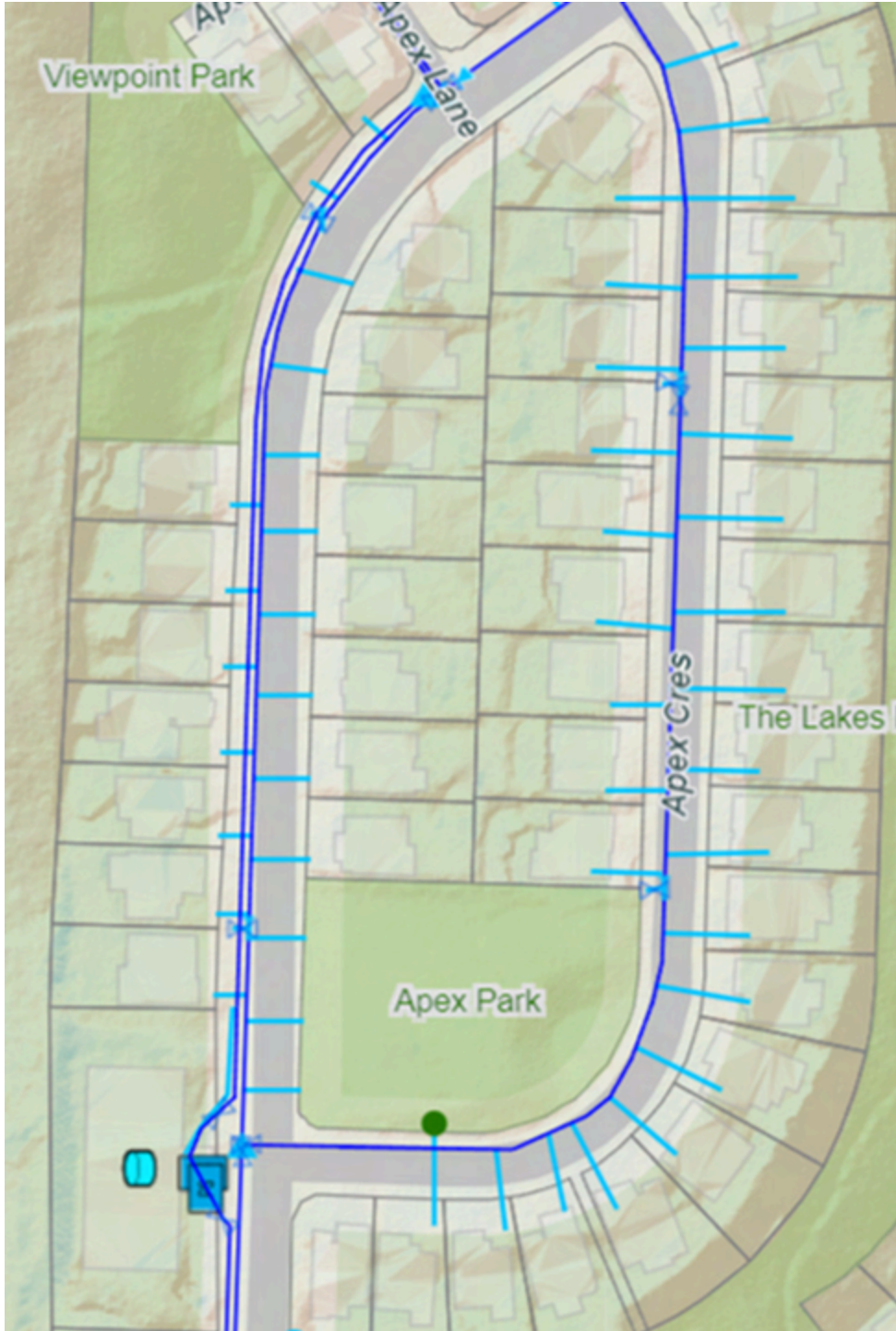
Figure 17: This map shows the water mains surrounding Apex Park (dark blue lines), along with the location of the water fitting (green dot) in the park (District of Lake Country, 2024a).
