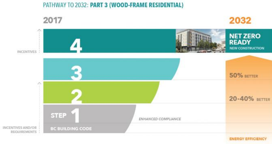
Figure 14: Four steps to achieve net-zero emission from Part 3 wood frame residential buildings (Energy Step Code 2018)
