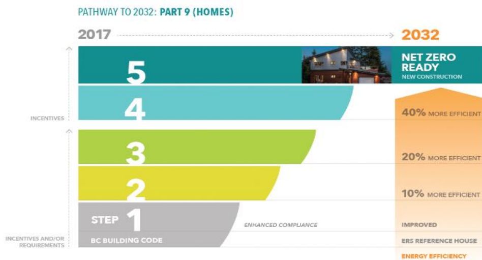
Figure 13: Five steps to achieve net-zero emission from Part 9 residential buildings (Energy Step Code 2018)
