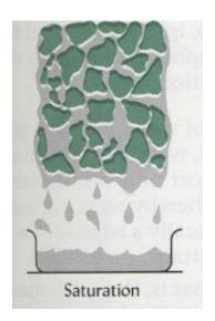
When all soil pores are filled with water  $(\psi_m \sim 0)$ , the soil is said to be saturated with water and it is at **maximum** retentive capacity
