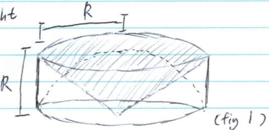
Cone  $(\frac{1}{3})(\text{area of base}) \times \text{height} = (\frac{1}{3})(\pi R^2)R$
