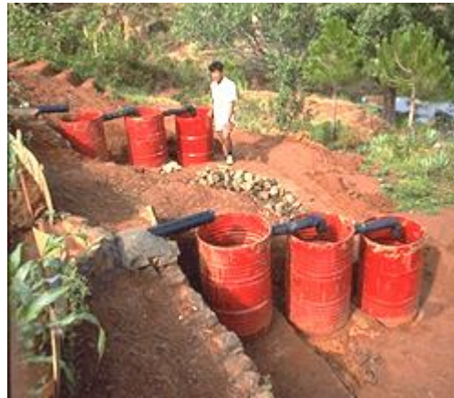
Photo 1. Example erosion plot covering 2 terraces (left) and the series of collection barrels at the base of the plot (right).
